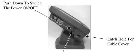
Slide Switch For Power On/Off Control
